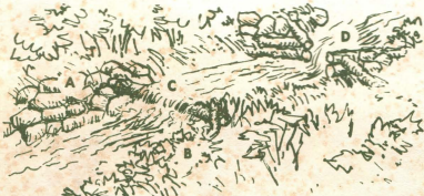
Stream Improvement Projects.—(A) Stone riprap, (B) streambank planting, (C) small log dam, (D) small V dam.
