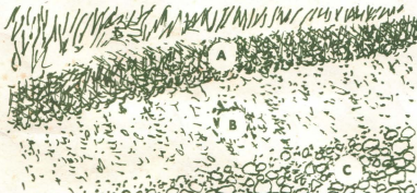
Soil Profile.—This cutaway section can teach how soil is formed and how it occurs in layers as (A) topsoil, (B) subsoil, and (C) parent soil.
